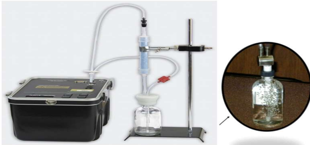
Fig. 2 Rad7 and Rad-H2o Set-Up for Radon in Water Detection.
